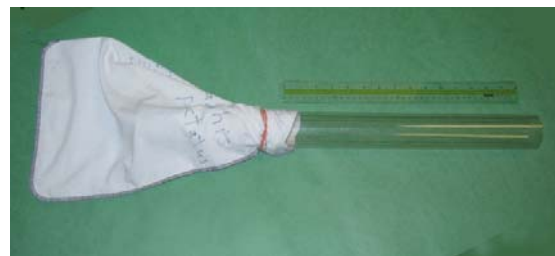
Figure 22. A 2-inch tube attached to a pillow case makes an excellent device to capture bats resting on walls. Photo by UNL.
