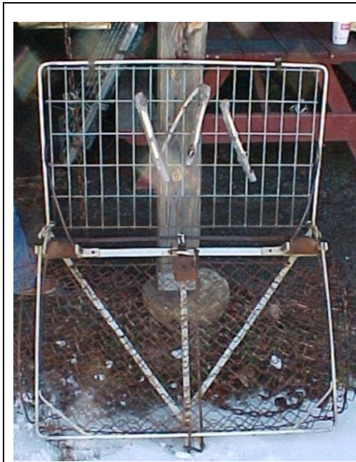
Figure 8. Demonstration set of a Hancock-style trap. Note sticks are for bait. Photo by Stephen M. Vantassel.
