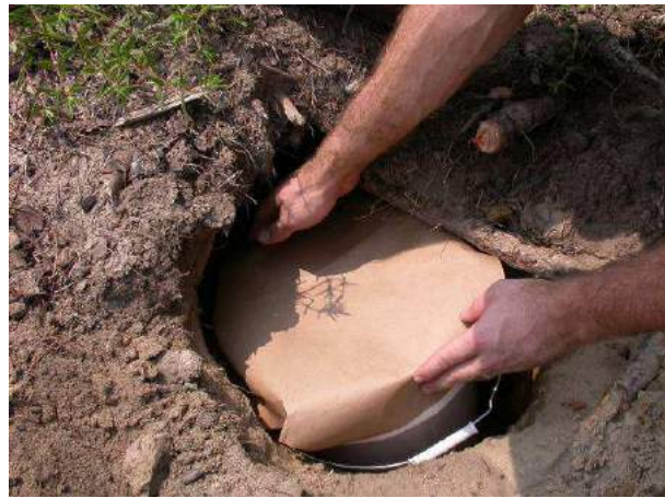
Packaging paper is fitted over bucket and folded around the edge.
