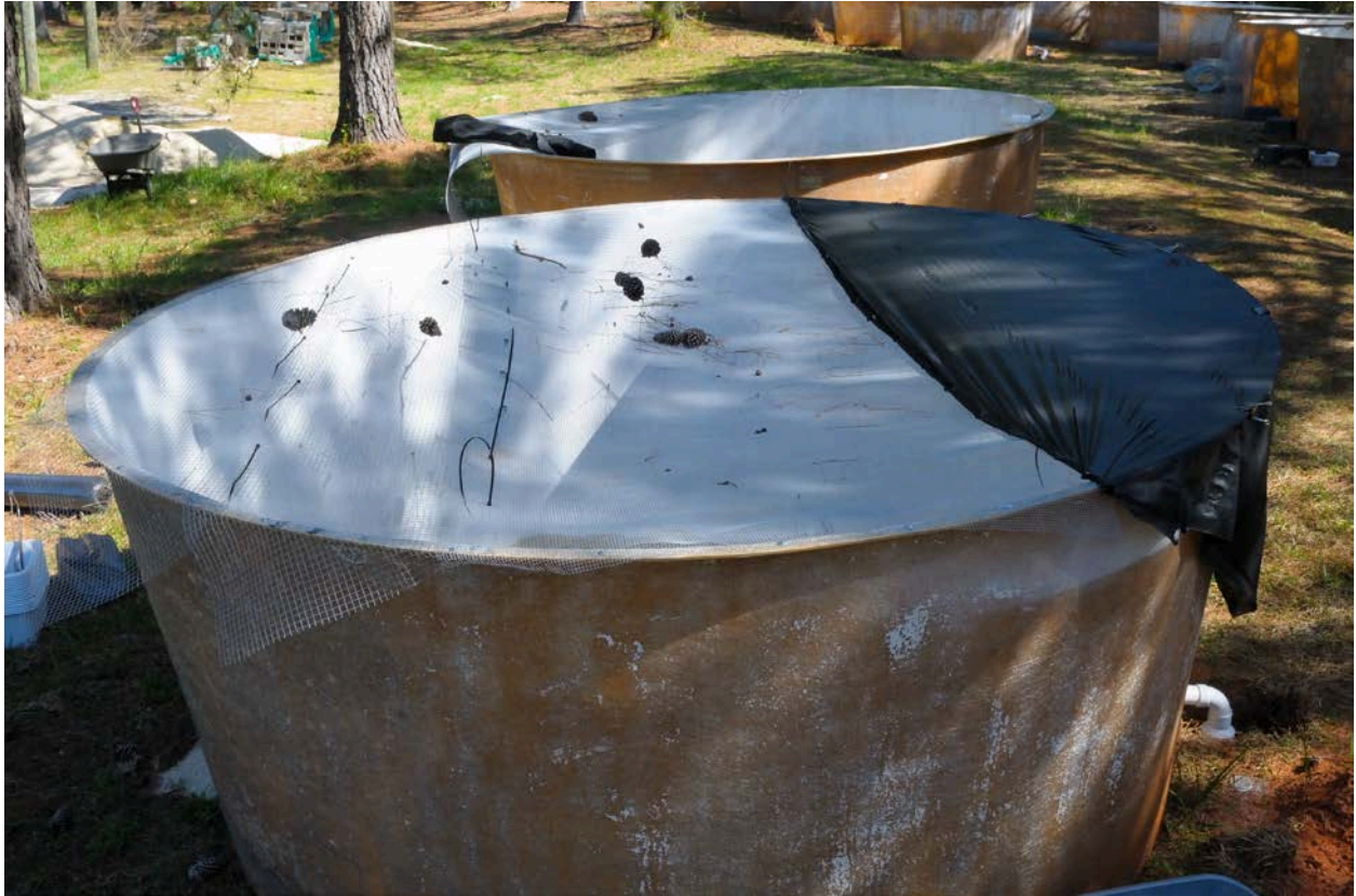
Figure 23. Hardware cloth and plastic ground cloth used as coverings of the tubs. The black plastic ground cloth served as a shade and door for access into the tubs.
