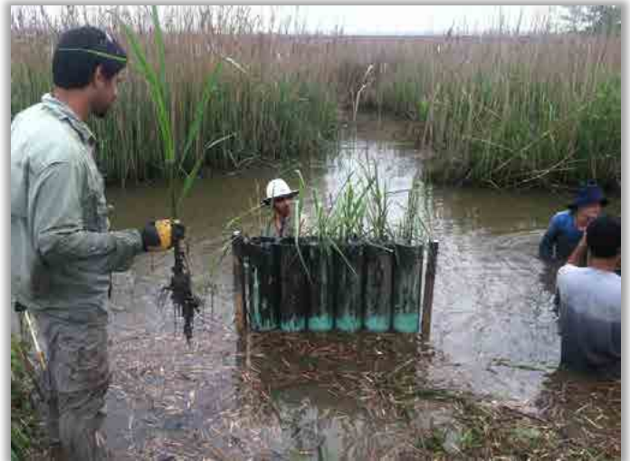
Marsh organs are used to study the effects of sea level rise on plant communities
